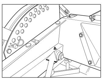
Lubricating the cutting height adjuster
